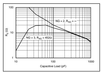
FIGURE 13. Required R<sub>S</sub> vs Noise Gain.
