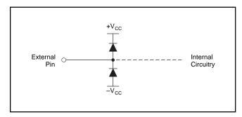
FIGURE 14. Internal ESD Protection.
