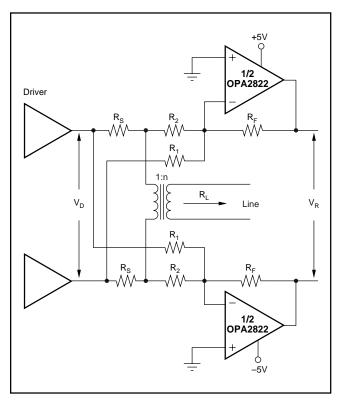
FIGURE 5. Example ADSL Receiver Amplifier.
