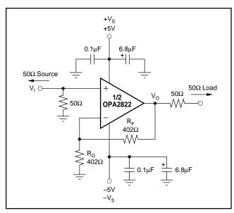
FIGURE 1. Noninverting G = +2 Specification and Test Circuit.
