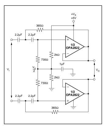
FIGURE 8. Single-Supply, 2nd-Order High-Pass Active Filter.
